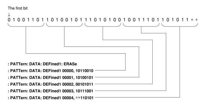
After the data are written, the first delivery address is set to "00000" and the data bit length is set to 38 bits before the delivery.
