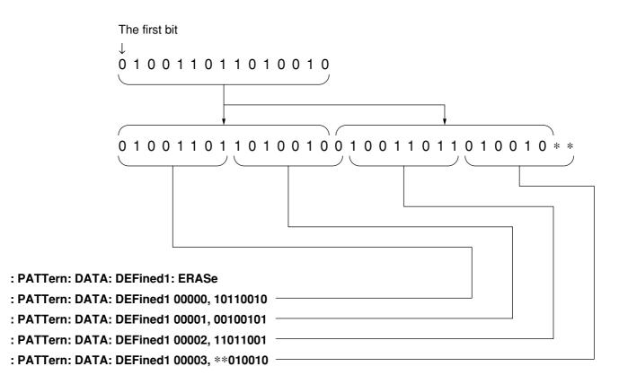
After the data are written, the first delivery address is set to "00000", the data bit length is set to 30-bits (15 bits×2), and the delivery method is set to 2-bit NRZ output before the delivery.
