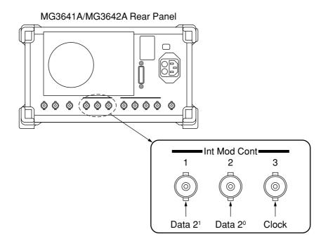
By sticking the attachment labels on near connectors, the erroneous wiring to the connectors can be prevented. Place the labels above the Int Mod Cont connectors as follows so that they can easily be seen (when the FSK encoder is implemented, stick its label adjacent to them):
