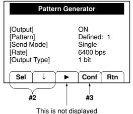
This is not displayed when the Pattern Generator output is set to OFF.
